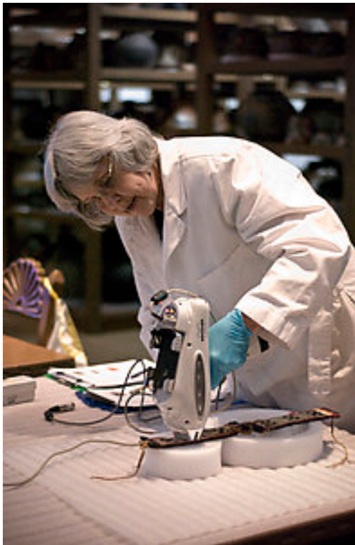
Conservator Cheryl Podsiki (Department of Anthropology, Field Museum) analyzing material culture with a non-destructive portable XRF spectrometer. ( https://sarweb.org/?symposium_native_collections_and_pesticides-p:symposiums )
